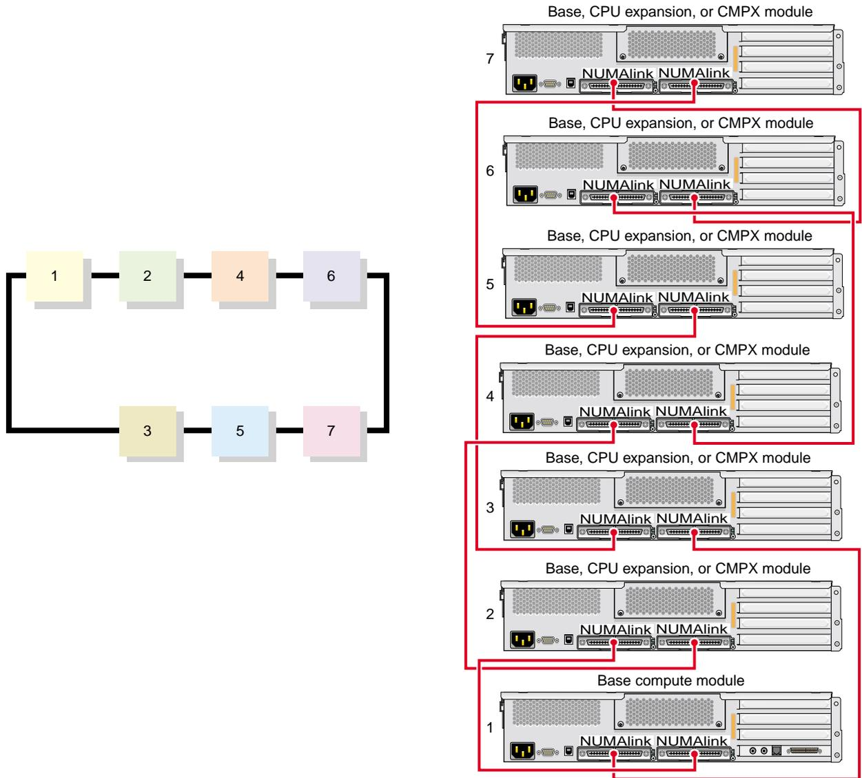
Figure 2-10 Seven Module Ring Topology
