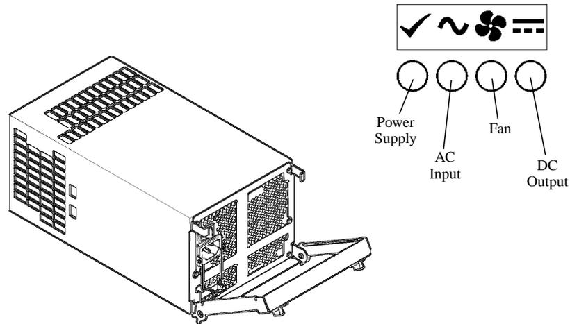
**Figure C-4** Power Supply/Cooling Module
