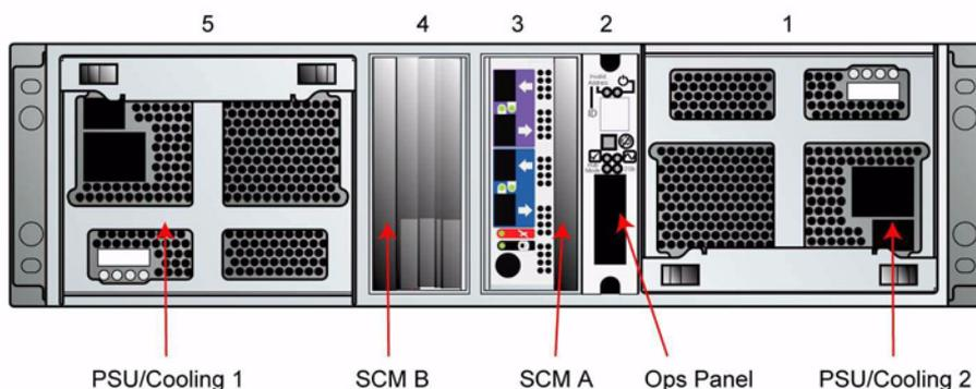
**Figure 5-3** Enclosure Chassis (Rear)
