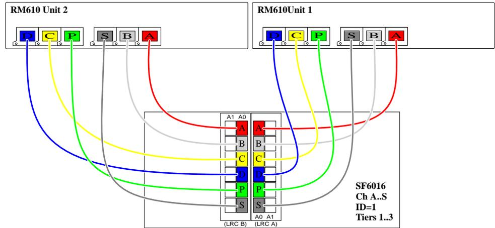
**Figure C-33** Connecting the SF6016 Enclosure to the RM610
