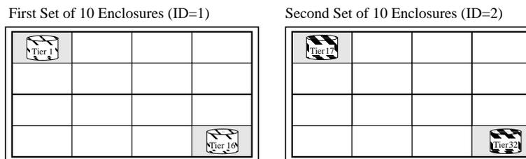
**Figure C-42** Drive Bays on SF2016 Enclosures for SES Communication Paths
