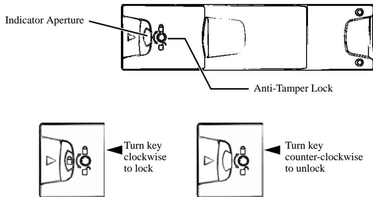
**Figure C-10** Anti-Tamper Lock on Drive Modules
