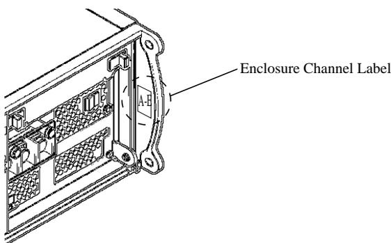
**Figure C-21** Enclosure Label at Rear
