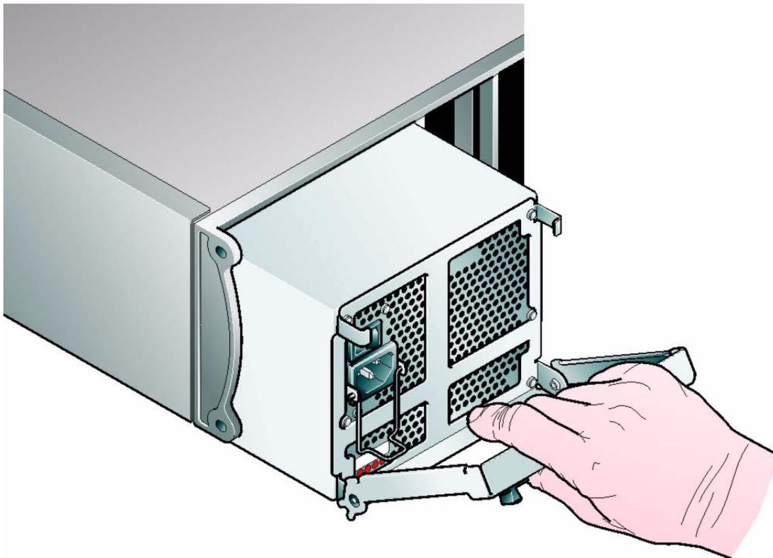
**Figure 8-4** Removing/Inserting an AC Power Supply/Cooling Module (3)
