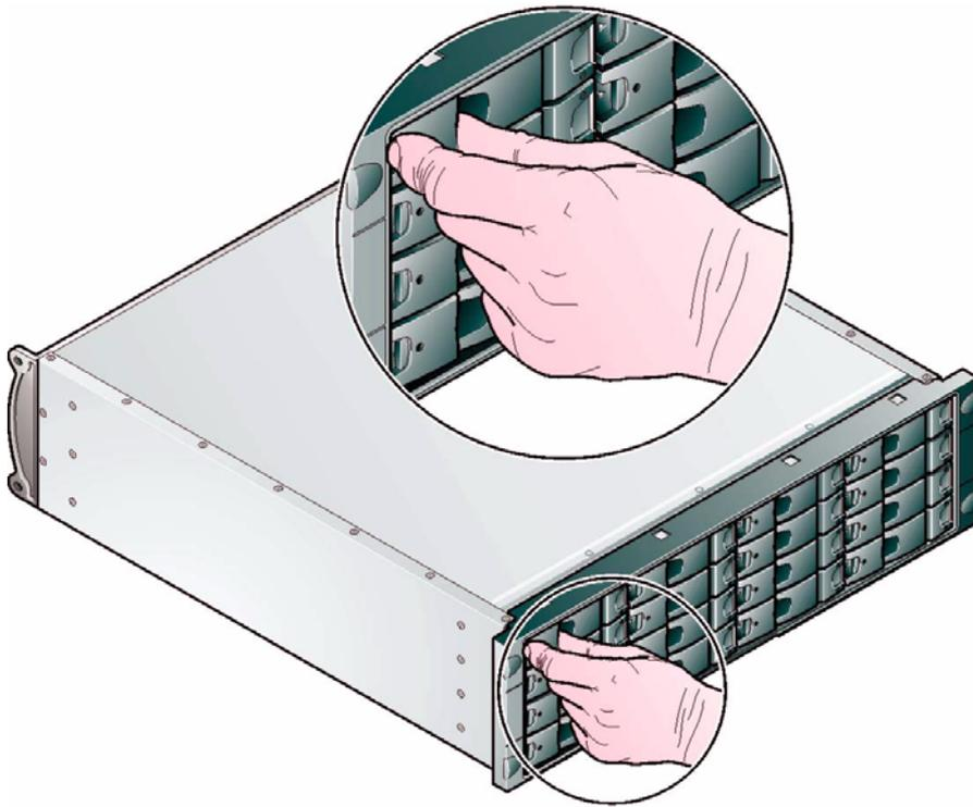
**Figure 6-19** Installing an SATA Drive Carrier Module (3)
