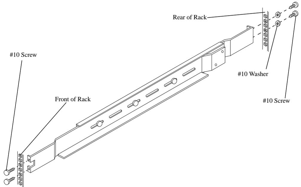
**Figure C-12** Fastening Rail/Support Assembly to Square/Through-Hole Rack (Left Hand Side)
