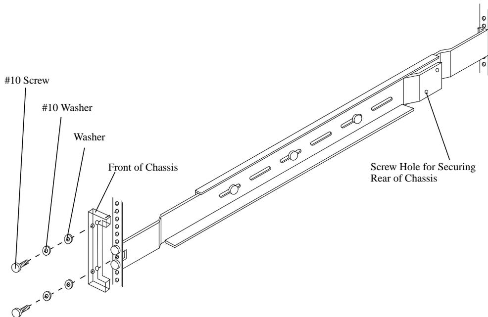
**Figure C-16** Securing Chassis to Threaded-Hole Rack (Left Hand)
