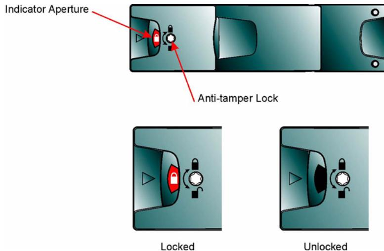
**Figure 5-10** Anti-tamper Lock
