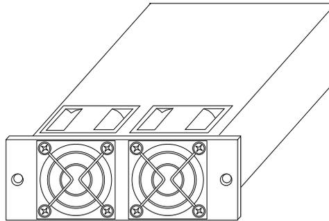
**Figure 1-7** Fan Module
