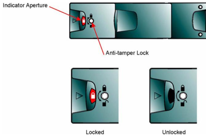
**Figure 6-20** Activating the Anti-tamper Lock
