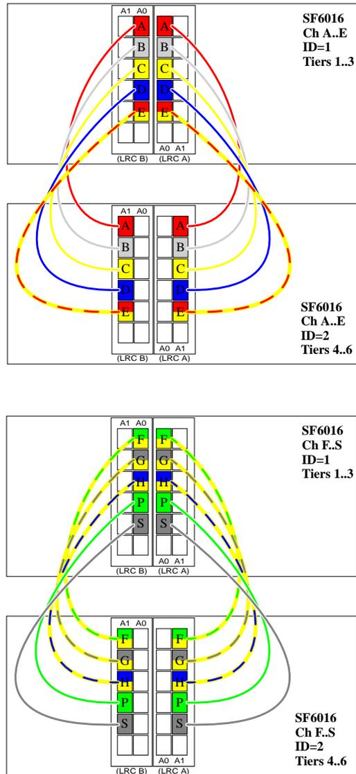
**Figure C-23** Daisy-Chaining the SF6016 Enclosures
