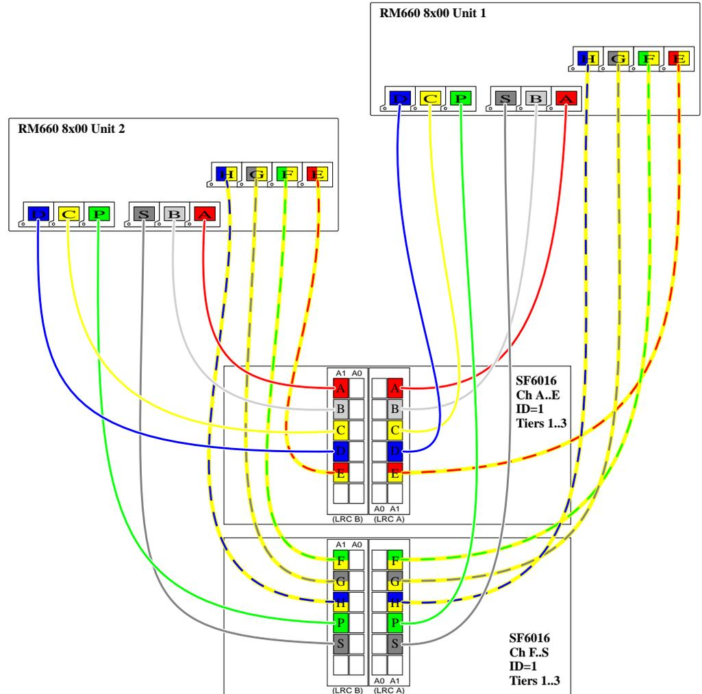
**Figure C-22** Connecting the SF6016 Enclosures to RM660
