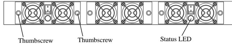
**Figure 4-2** Power Supply/Cooling Modules in the Front of the RM610
