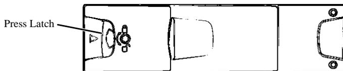
**Figure C-14** Latch Operation on Drive Module
