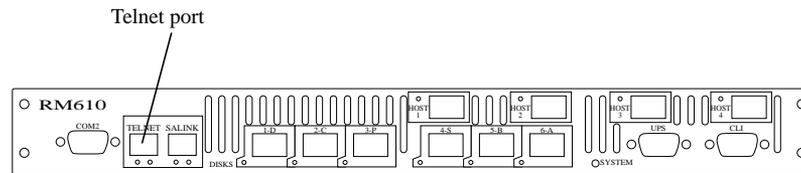
**Figure 3-72** Telnet Port on the RM610
