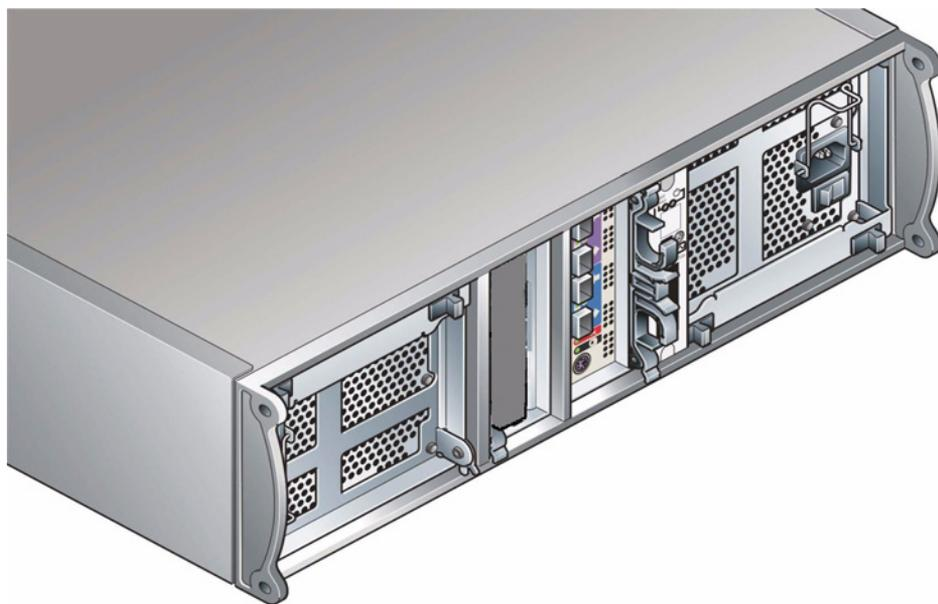
**Figure 5-8** SA2016 System Enclosure with LRC I/O Modules Installed
