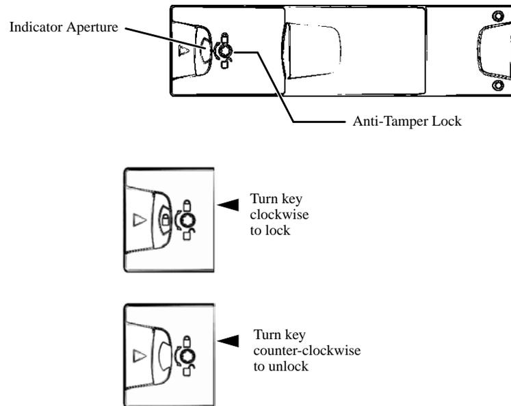
**Figure C-45** Activating the Anti-Tamper Lock
