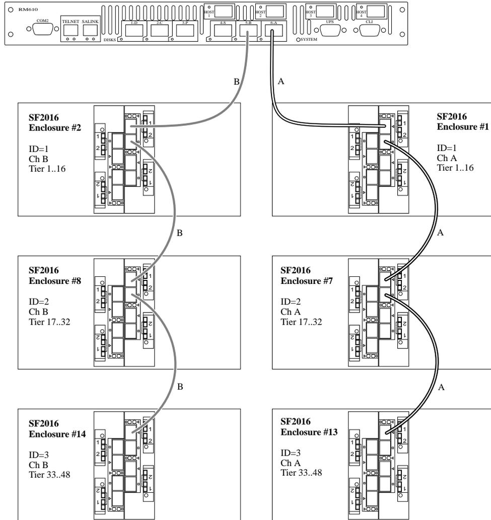
**Figure C-40** Daisy-Chaining the SF2016 Enclosures
