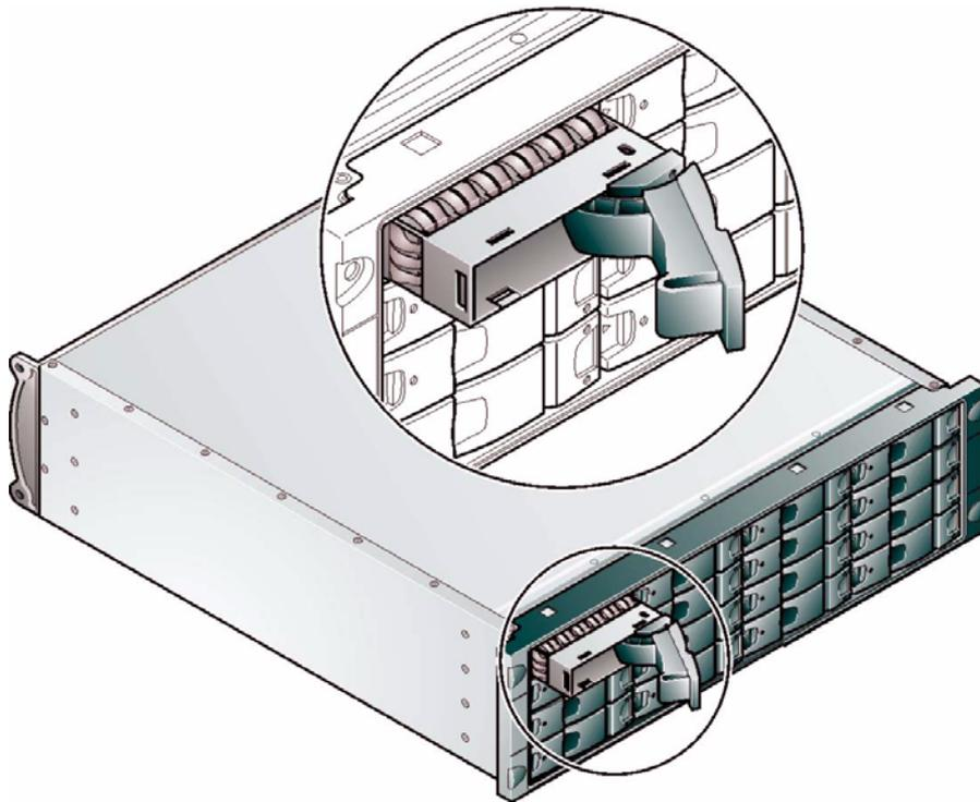
**Figure 6-18** Installing a SATA Drive Carrier Module (2)
