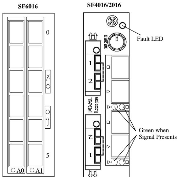
**Figure C-7** I/O Module Connectors and LEDs
