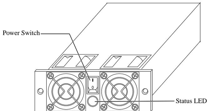
**Figure 1-2** Power Supply/Cooling Module
