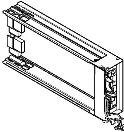
**Figure C-5** FC-AL LRC I/O Module
