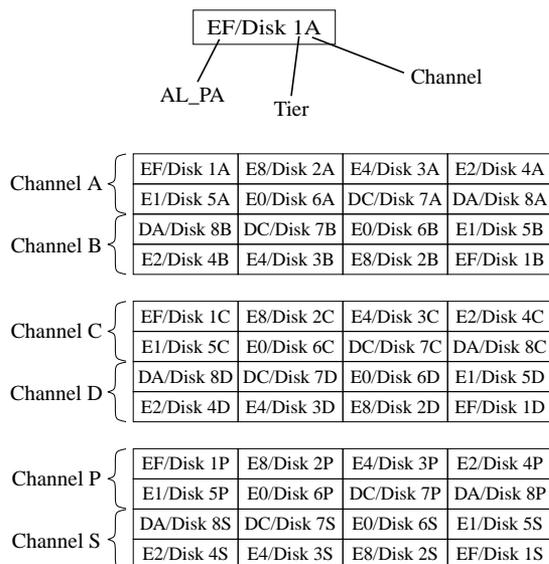
**Figure 2-15** Channel and Tier Numbering of Drives on SF4016 Enclosures
