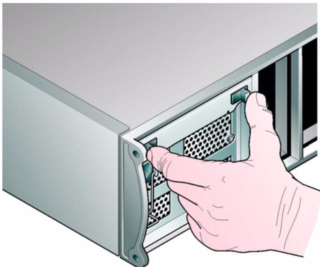
**Figure 6-4** Installing an AC Power Supply Cooling Module (2)
