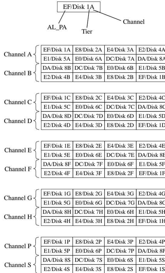
**Figure 2-14** Channel and Tier Numbering of Drives on SF4016 Enclosures
