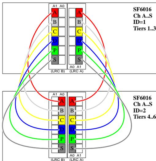
**Figure C-34** Daisy-Chaining the SF6016 Enclosures
