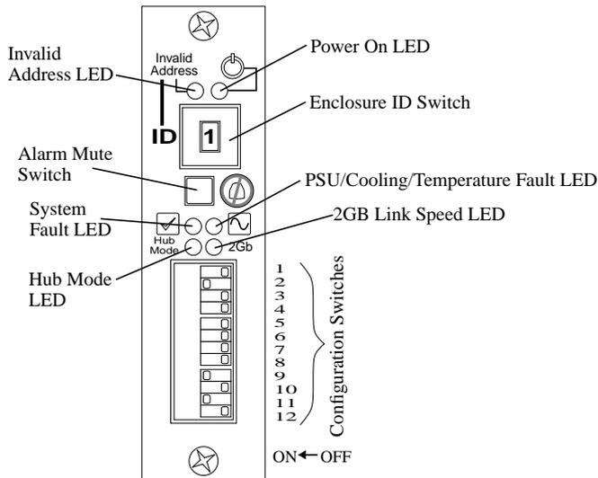
**Figure C-47** Ops Panel LEDs
