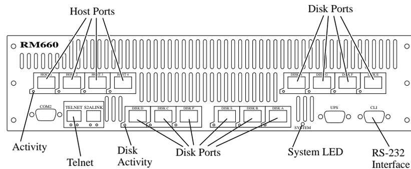
**Figure 1-4** I/O Ports on Rear Panel of the RM660
