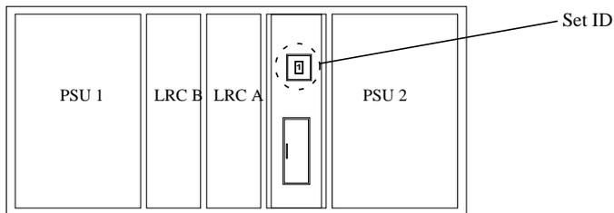
**Figure C-35** Enclosure ID Switch
