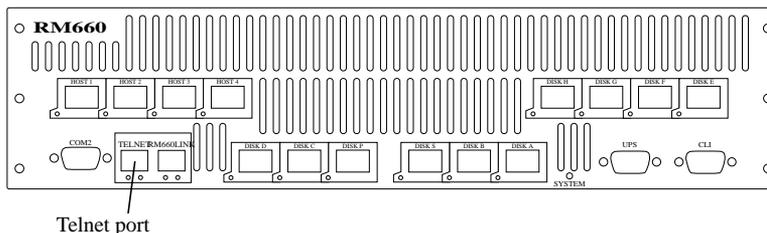
**Figure 3-71** Telnet Port on the RM660
