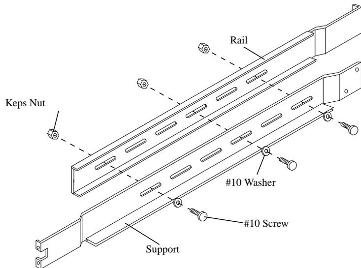
**Figure C-11** Assembling Rail to Support (Left Hand Assembly)
