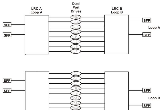
**Figure C-6** Overall Loop Layout
