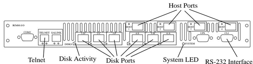
**Figure 1-8** I/O Ports on Rear Panel of RM610
