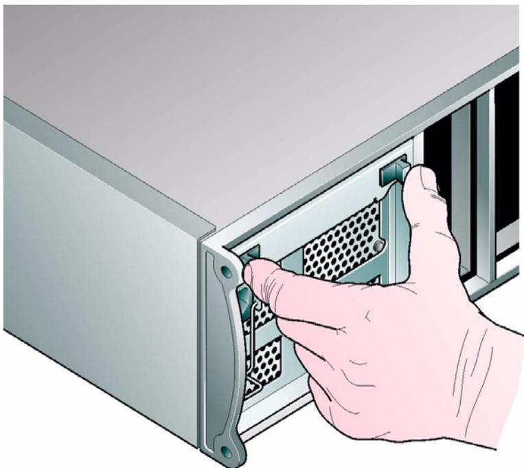
**Figure 8-2** Removing/Inserting an AC Power Supply/Cooling Module (1)
