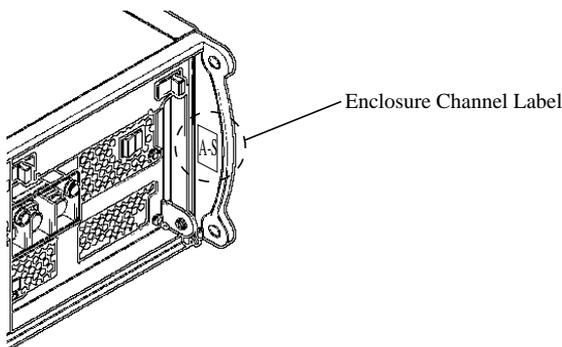
**Figure C-32** Enclosure Label at Rear
