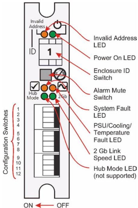
**Figure 7-1** Ops Panel LEDs and Switches
