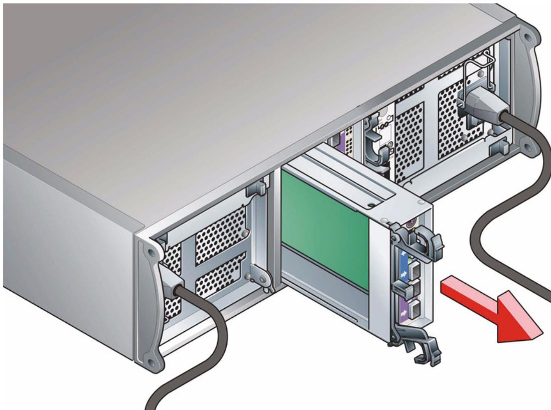
**Figure 8-6** Removing an LRC I/O Module (2)
