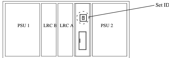
**Figure C-24** Enclosure ID Switch
