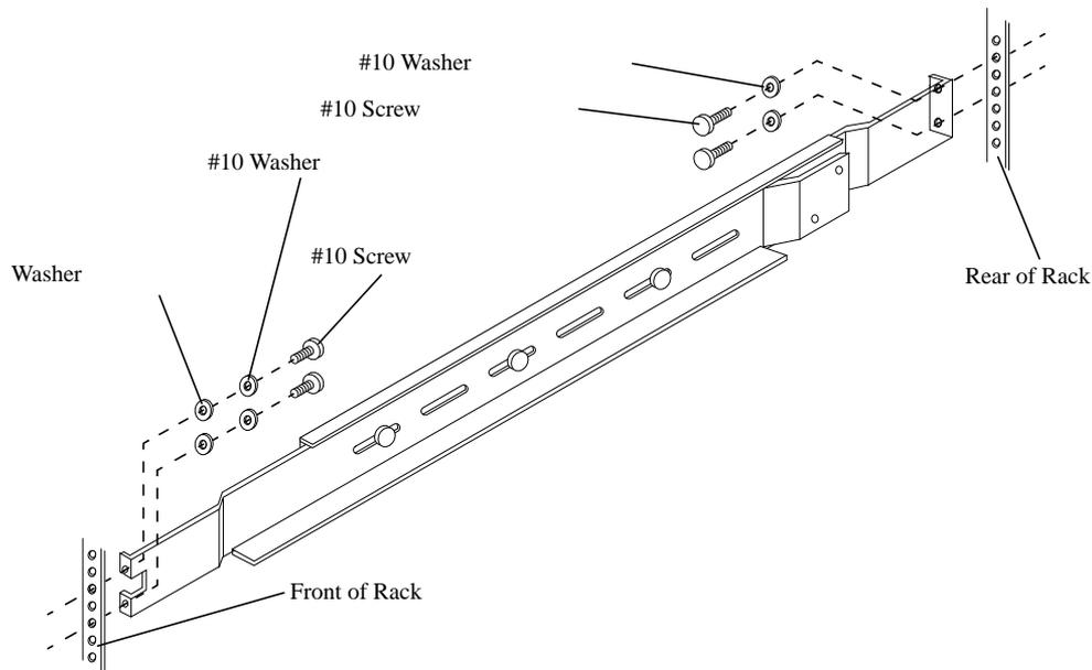
**Figure C-13** Fastening Rail/Support Assembly to Threaded-Hole Rack (Left Hand Side)
