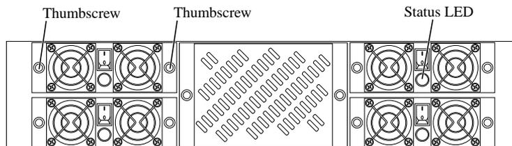
**Figure 4-1** Power Supply/Cooling Modules in the Front of the RM660
