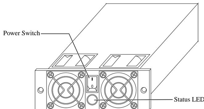
**Figure 1-6** Power Supply/Cooling Module
