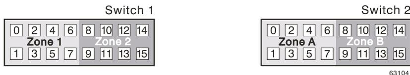
**Figure 3-27** Switch Zoning for the Intra-Site Configuration
