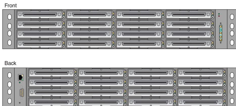
**Figure 5-2** Dense Router Module Front and Rear Panels
