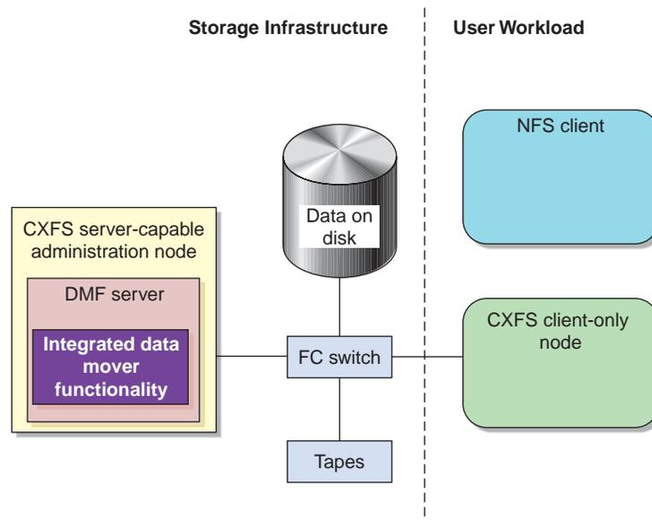
**Figure 1-4** Basic DMF in a CXFS Environment
