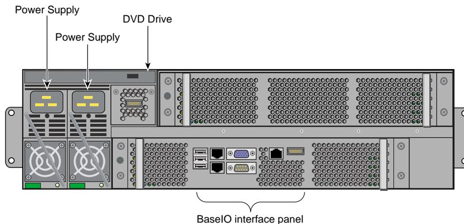
**Figure 1-4** SGI Altix UV 100 IRU Front View
