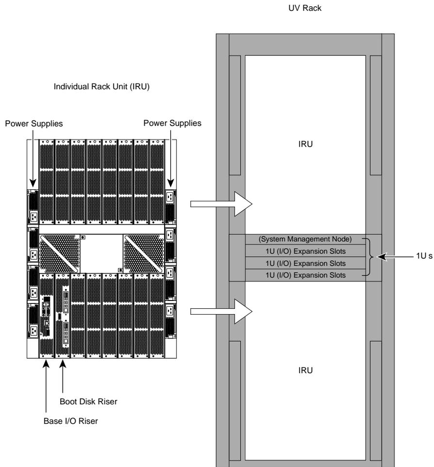
**Figure 1-2** Basic System Building Blocks for Altix UV 1000 Systems
