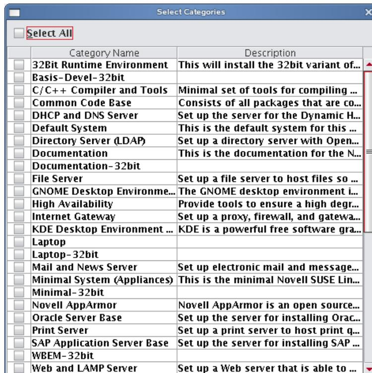
12. Select which payload categories to install or remove by clicking the checkbox next to each package.
