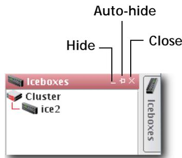
**Frames** — Provide you with specific control over common aspects of cluster systems (for example, imaging and user accounts). Each frame tab opens a frame containing a navigation tree that allows you to manage system components easily. The navigation tree is found in most frames and is used to help organize cluster components. You may dock, close, or relocate frames and frame tabs as needed.
