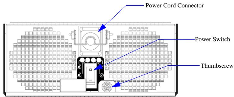
4. Ensure that the power switch on the new (replacement) module is OFF.
