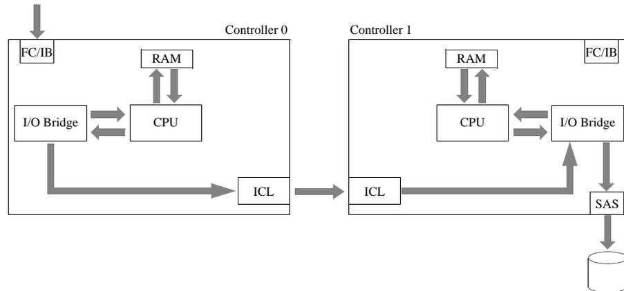
Properly configured and tested host side multi-path drivers will ensure right side I/O will occur. If poor performance is encountered, especially upon initial configuration, then verifying and correcting your primary path to disks is essential.
