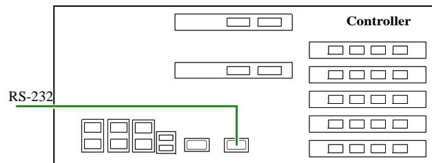
2. Load a serial console program (such as HyperTerminal, minicom, and screen) and use the following settings for the serial connection:
