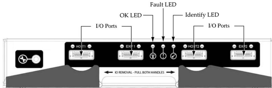
The four I/O ports provide connections to the IS16000 Controllers. The various LED indicators are listed in Figure 25.
