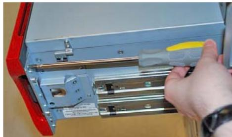
3. Once the front bezel is removed, it is possible to see the piano switches through the grey bezel (Figure 36). If the switches are hidden by a Mylar switch cover, remove the cover with a small pair of tweezers. If the switches are still not visible, remove the grey bezel. It is attached to the chassis with 32 small screws (18 on the front and 14 on the bottom).
