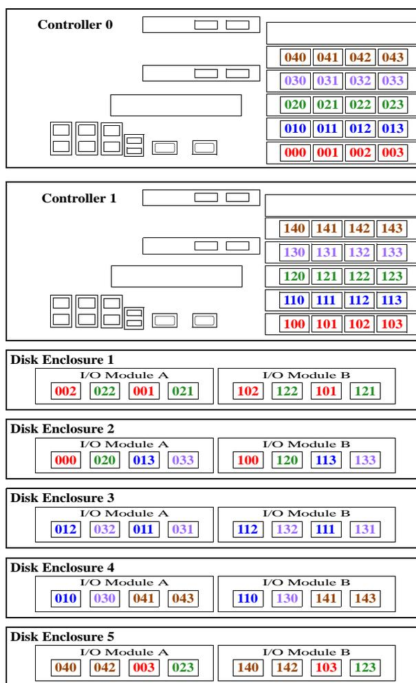
Figure 39. Connecting 5 Disk Enclosures (with SATA and SAS Disks) to Controllers
