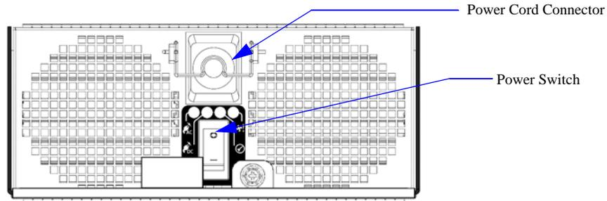
The disk enclosure must always be operated with two PCM installed. Module replacement should only take a few minutes to perform but must be completed within 5 minutes from removal of the failed module. Four (4) LEDs mounted on the PCM indicate the status of the module and the fans (Figure 22). Figure 23 provides a description of the color and status of the LEDs.
