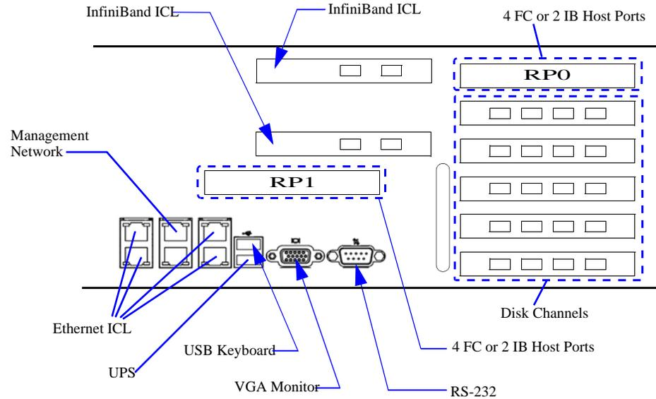
The InfiniBand ICL and Ethernet ICL ports provide connections for Mirrored Write Back Cache and control between the Controllers in a couplet configuration.
