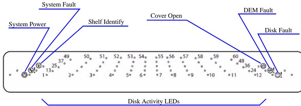
Figure 19. Front Panel LED Description
