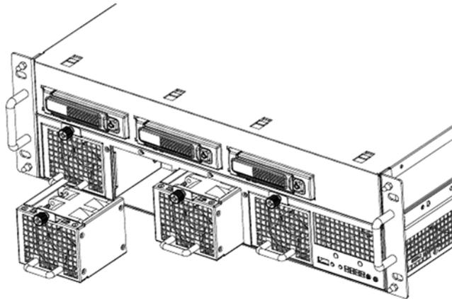
4. Slide the new fan into the bay, making sure that it is fully inserted.
