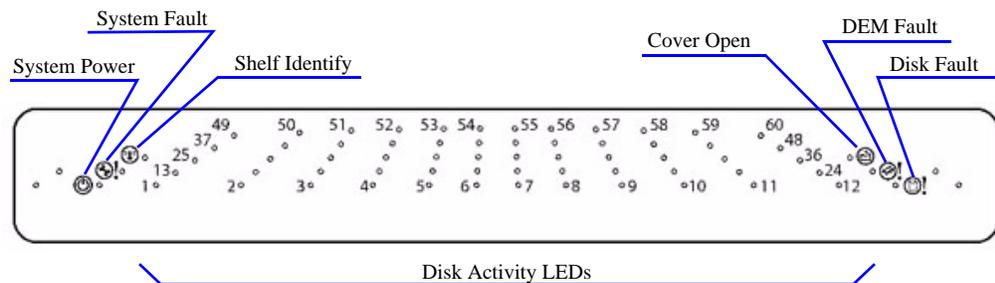
Figure 138. Front Panel LED Description
