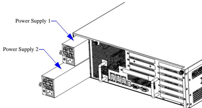
4. Slide the replacement module into the bay, making sure that it is fully inserted.
