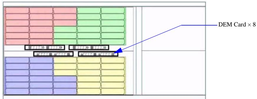
Each DEM (Figure 28) connects to a single port of the HDD based on the location within the enclosure within which it is installed. Each card provides power control signals to each disk slot. It controls HDD identify/service LEDs and monitors the status from partner DEM. Each pair of DEMs supports 15 disk modules.
