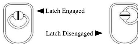
3. On the disk module, slide the latch backward to release the handle (Figure 34).
