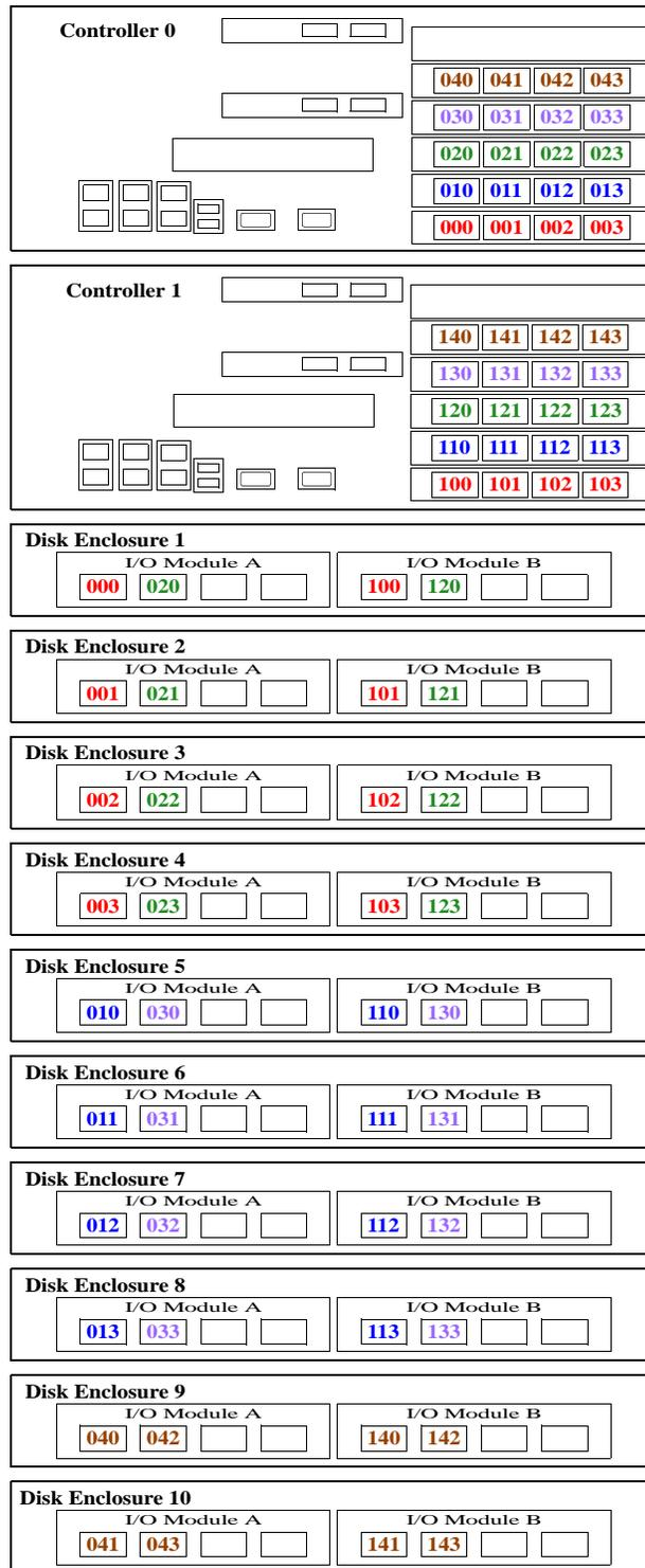
Figure 41. Connecting 10 Disk Enclosures (with SATA and SAS Disks) to Controllers
