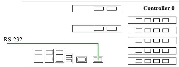
2. Load a serial console program (such as HyperTerminal, minicom, and screen) and use the following settings for the serial connection:
