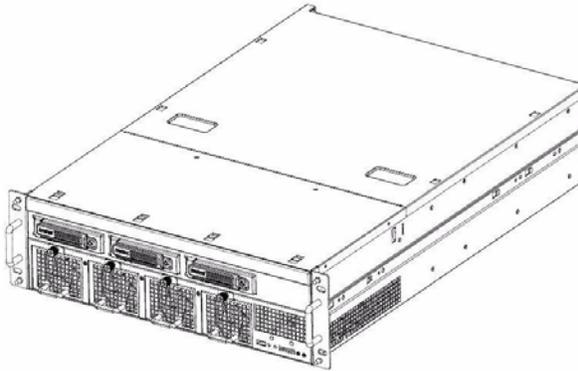
At the front, there are four fan modules, three internal disk modules, control buttons and status LED indicators (Figure 3).
