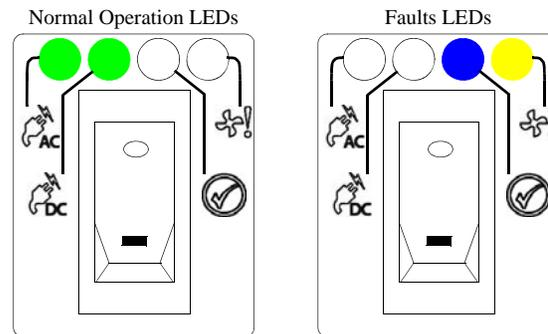
Figure 23. disk enclosure PCM LED Description
