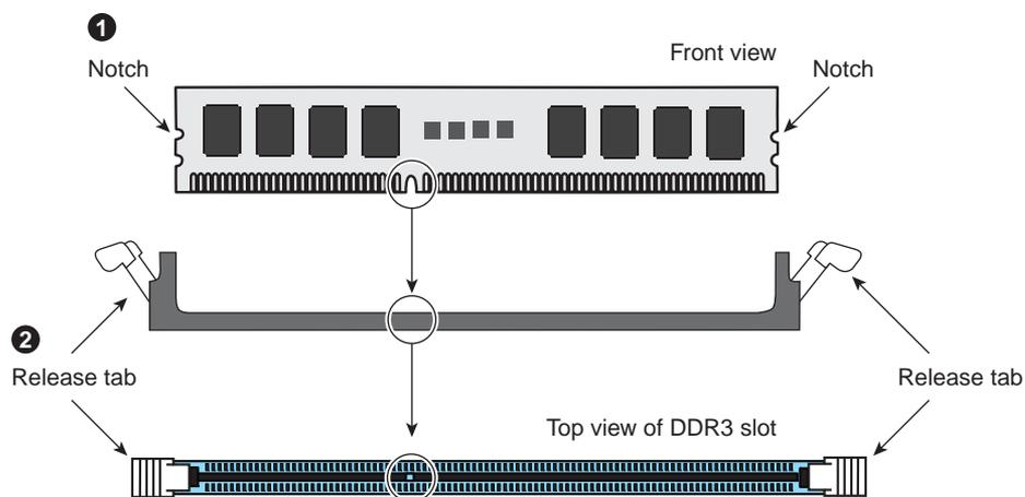
**Figure 5-4** DIMM Installation Example
