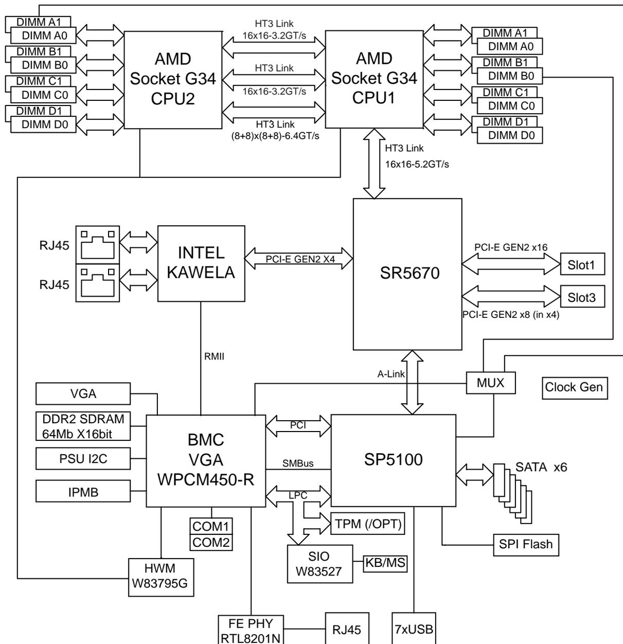
**Figure 1-2** Processor and I/O Chipset System Block Diagram
