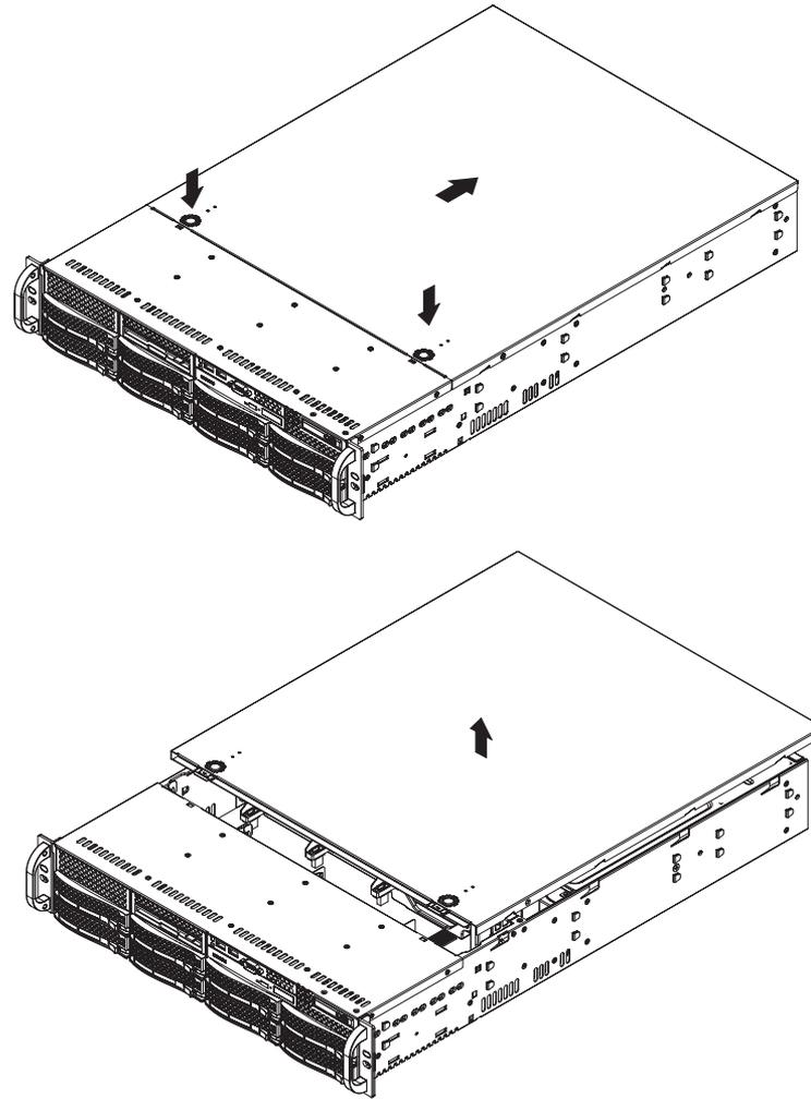
**Figure 2-4** Accessing the Inside of the System
