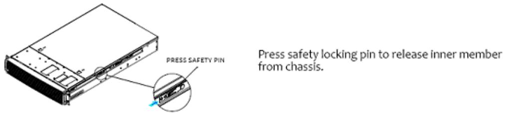
**Figure 4-17** Removing the Inner Member from the Chassis
