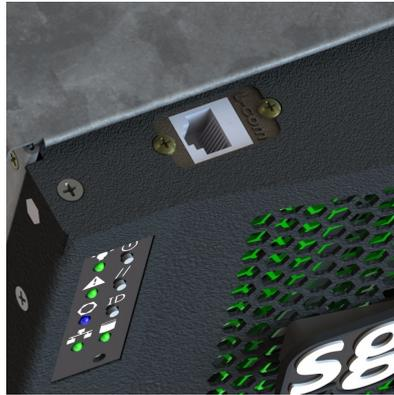
**Figure 1-60** MIS-S9D Proprietary Network Interface
