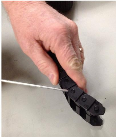
**Figure 1-45** Remove Segments from the End of an Empty Arm
