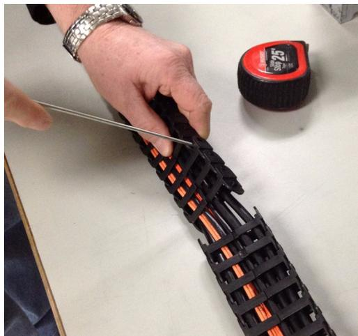
**Figure 1-52** Pry Apart the Joint at the Other End
