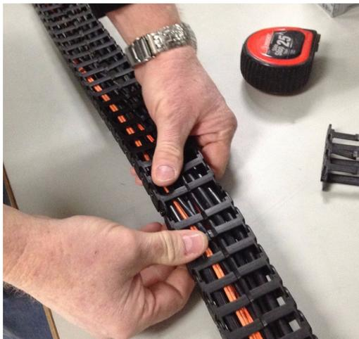
**Figure 1-54** Join the Spliced Ends of the Cable Management Arm
