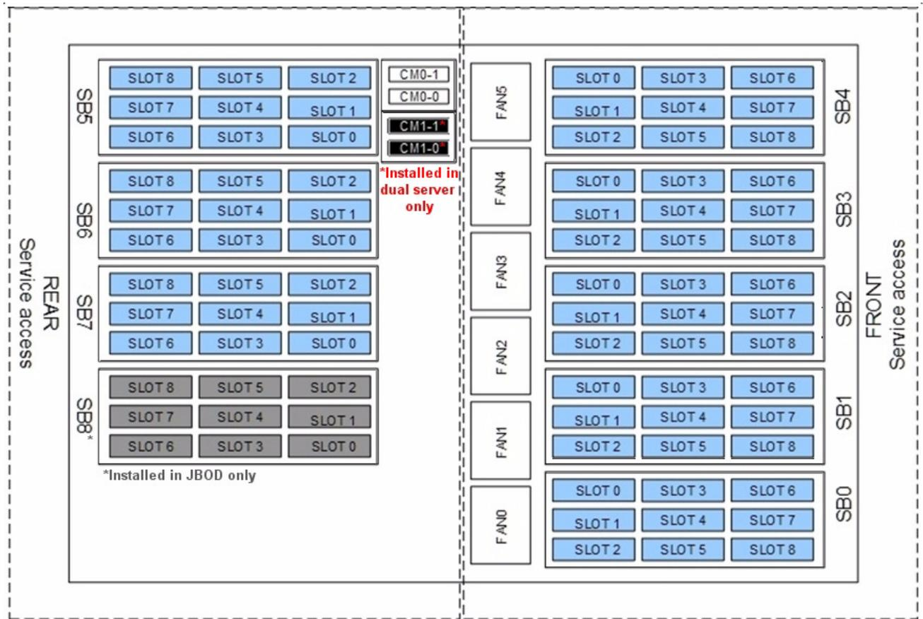
**Figure 1-23** System Layout Diagram – Drive & Fan Placement
