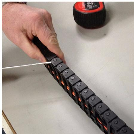
**Figure 1-49** Remove Segments from the Middle of a Full Arm
