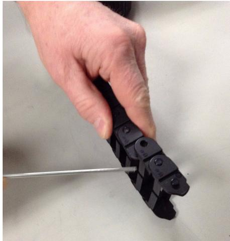
**Figure 1-46** Pry the Joint Apart
