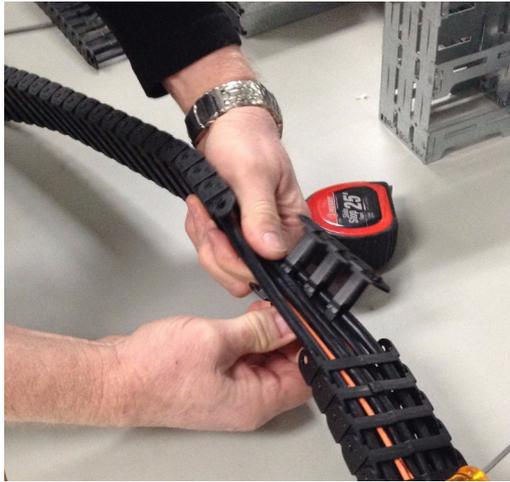
**Figure 1-53** Twisting the Section of Segments from the Cables
