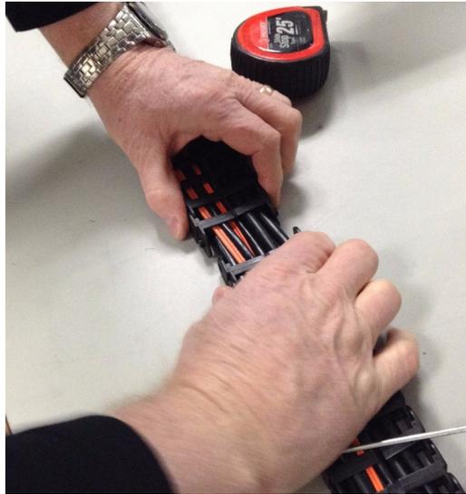
**Figure 1-51** Pull Apart the Cable Management Arm
