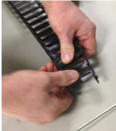
**Figure 1-47** Pull the Segments from the Arm
