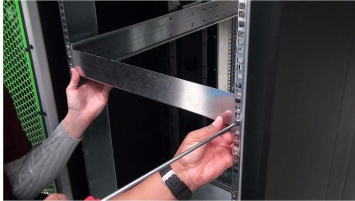
**Figure 1-15** Adjustment Using the Alignment Tool
