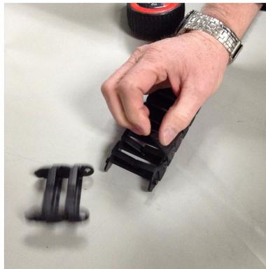
**Figure 1-51** Shortened Arm Ready for Installation
