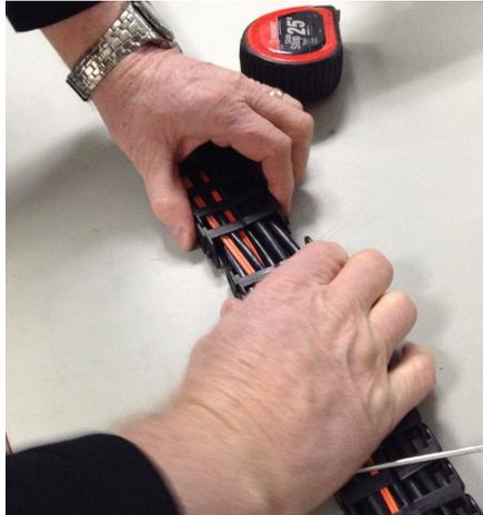
**Figure 1-54** Pull Apart the Cable Management Arm
