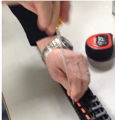
**Figure 1-53** Pry Open the Segment Joint
