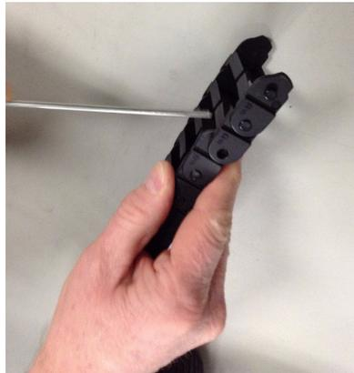
**Figure 1-49** Pry the Joint Apart
