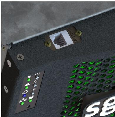
**Figure 1-76** MIS-S9D Proprietary Network Interface
