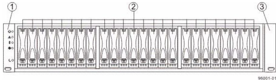
1. Left End Cap (Has the Drive Tray LEDs)
