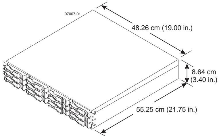
**Figure 35 Dimensions of the E5500 Controller-Drive Tray (24-Drive Model) – Front View**
