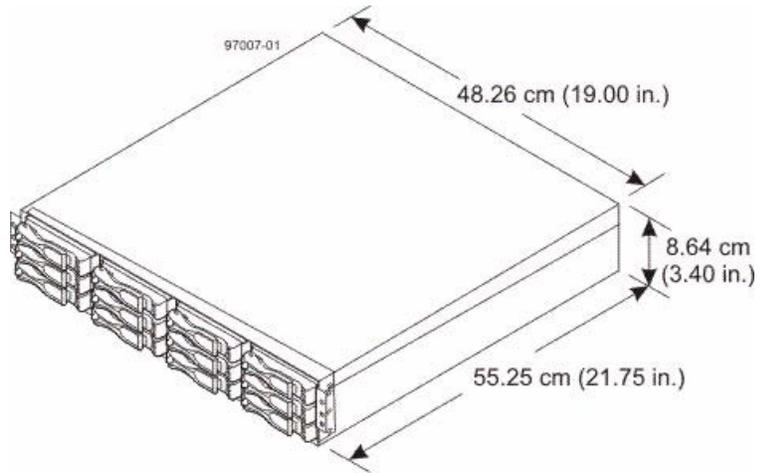
**Figure 13 Dimensions of the E2600 Controller-Drive Tray (24-Drive Model) – Front View**
