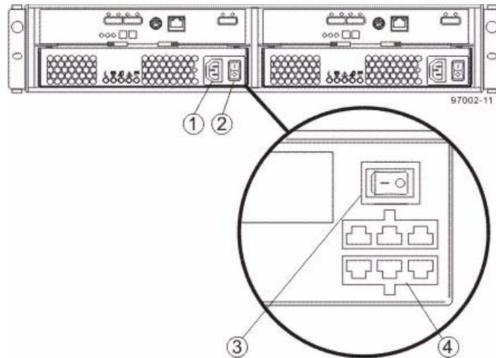
1. AC Power Switch on the AC Power-Fan Canister
