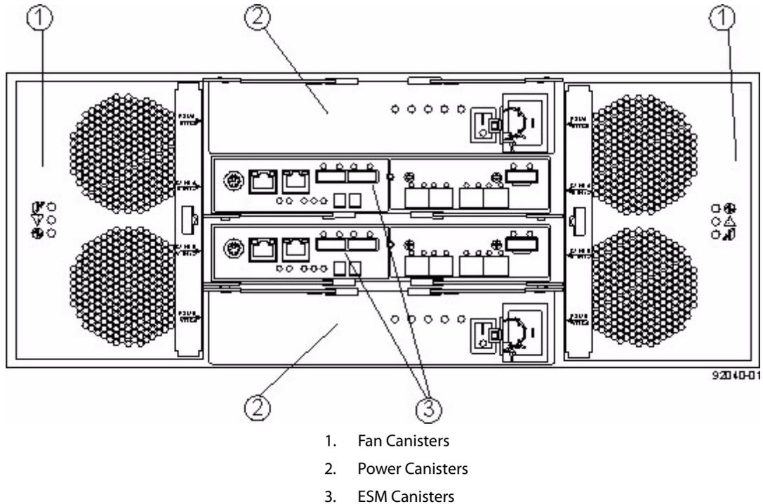
An AC power source supplies power to the power canister.
