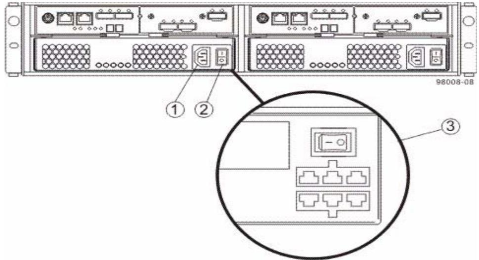
1. AC Power Connector on the AC Power-Fan Canister
