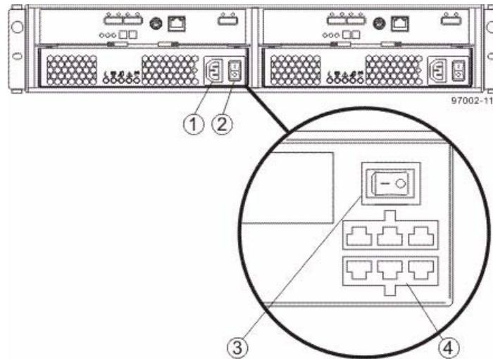
1. AC Power Connector on the AC Power-Fan Canister
