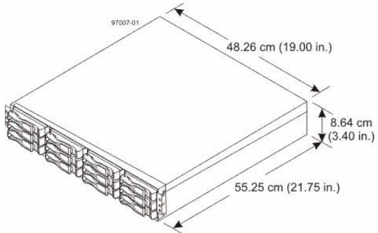
**Figure 24 Dimensions of the E5400 Controller-Drive Tray (24-Drive Model) – Front View**
