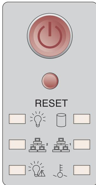
**Figure 3-1** System Front Control Panel Indicator Components
