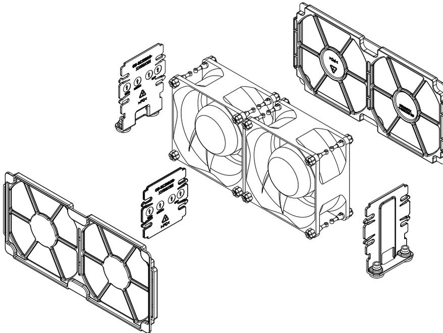
**Figure 6-8** Mid-chassis Fan Assembly Example
