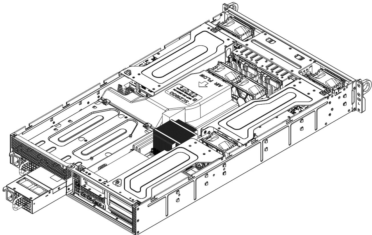
**Figure 6-4** Power Supply Remove/Replace Example
