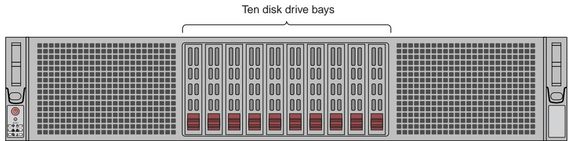
**Figure 5-3** C2110G-RP5-P System Disk Drive Locations
