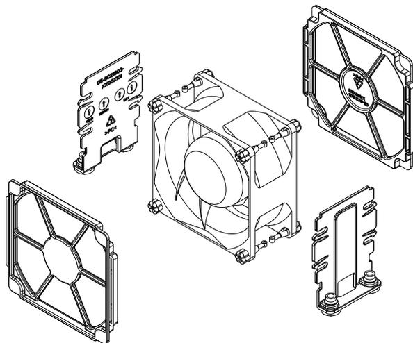
**Figure 6-9** Front/GPU Fan Assembly Example
