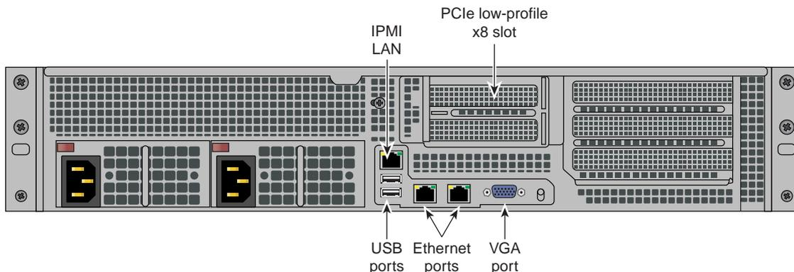
**Figure 6-10** Low-Profile PCIe Slot Location
