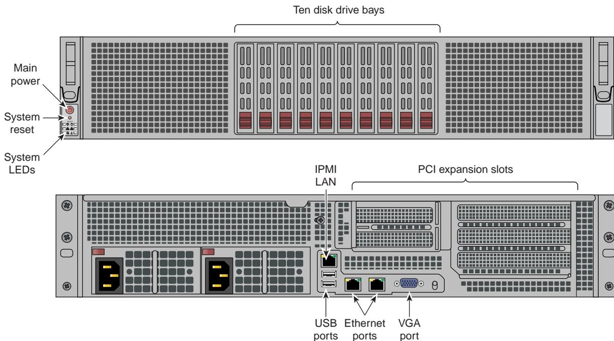
**Figure 1-1** Server Front and Rear View Examples
