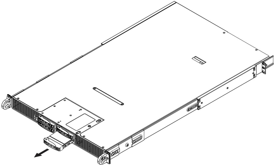
**Figure 6-2** Remove Drive and Carrier from Front of Server
