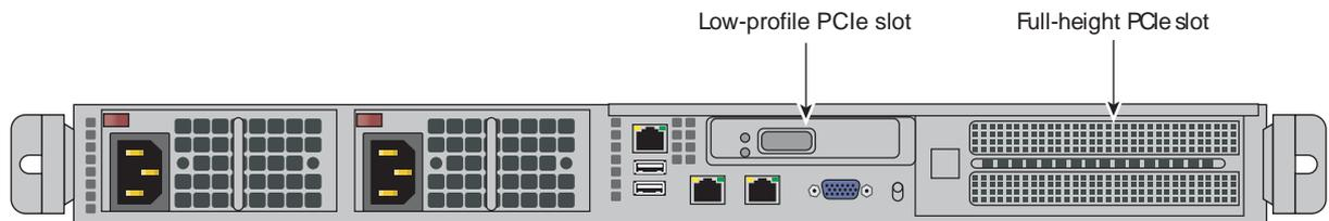
**Figure 6-9** Rear PCIe Low-profile and Optional Full-height Slot Locations
