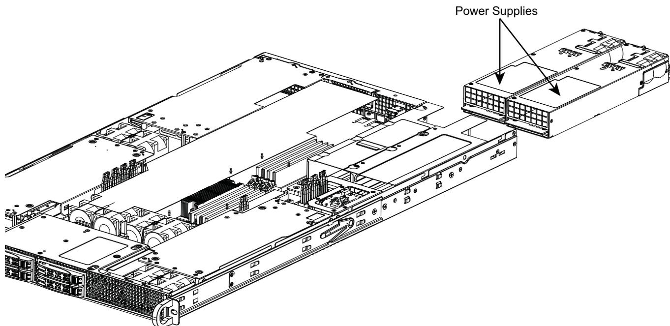
**Figure 6-5** Power Supply Remove/Replace Example
