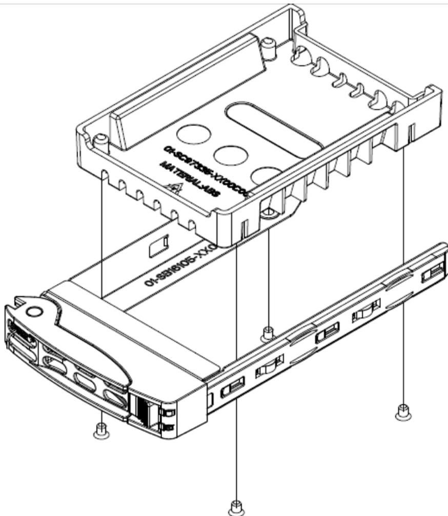
**Figure 6-3** Drive Carrier Attachment to Dummy Drive Blank Example
