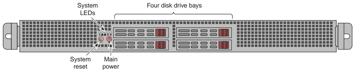
**Figure 5-3** C1104-GP1 System Disk Drive Locations
