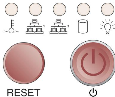
**Figure 3-1** System Front Control Panel Indicator Components
