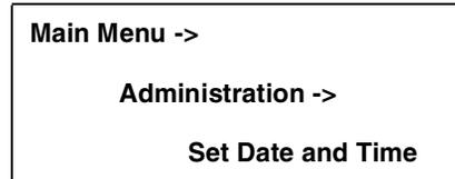
When the autoloader is initially set up, or if it has been unplugged for approximately 8 days, you need to set the date and time. If the date and time are not set, error logs will not include the date and time stamps.
