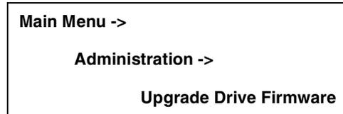
5. From the **Upgrade Drive Firmware** menu, use the [-] or [+] key to select the slot containing the firmware upgrade tape. Select **[OK]**.
