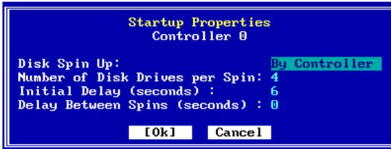
**Figure 2-9. Startup Properties Screen**
