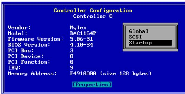
Figure 2-8. Properties Menu Overlays Controller Configuration Screen
