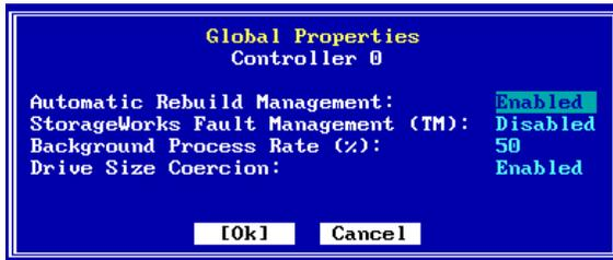
**Figure 2-5. Global Properties Screen - New Controllers**
