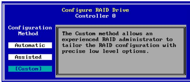
Figure 2-56. Configure RAID Drive - Custom
