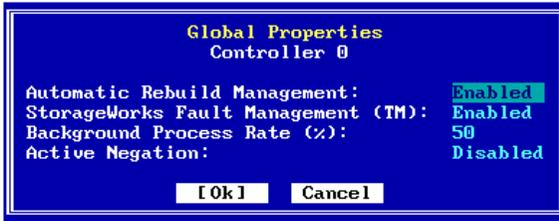
**Figure 3-4. Global Properties Screen - Previous Controllers**
