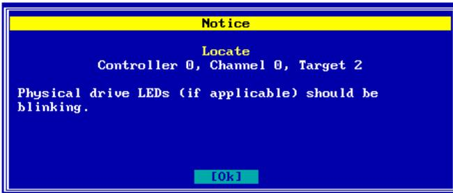
**Figure 4-73. Locate Physical Device Notice**
