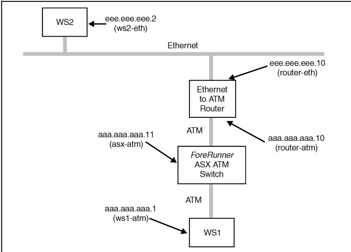
**Figure 4.2 - ATM Network with Access to Ethernet**
