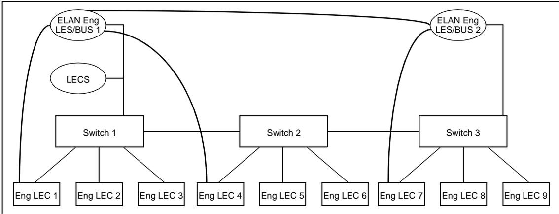
**Figure 7.16 - ELAN with Multiple Servers in Operation**
