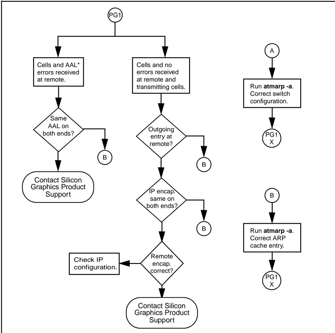
Figure 10.4 - Networking Connectivity Using PVCs (Page 2)
