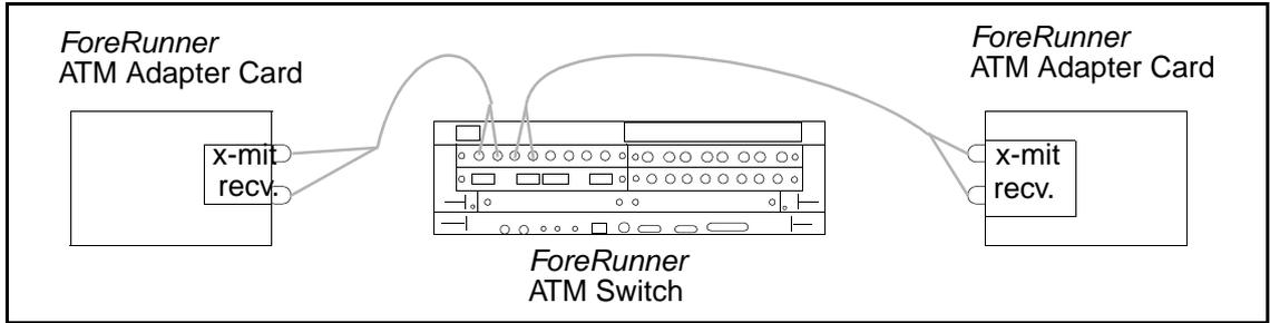
Figure B.1 - Minimum Configuration with UNI 3.0 or UNI 3.1 Signalling
