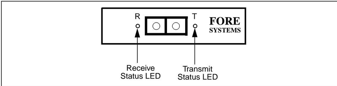
Figure A.1 - SC Connector Face Plate Configuration
