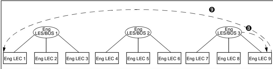
**Figure 7.11 - LE-ARP Response Delivered and LEC 9 Contacts LEC 1**
