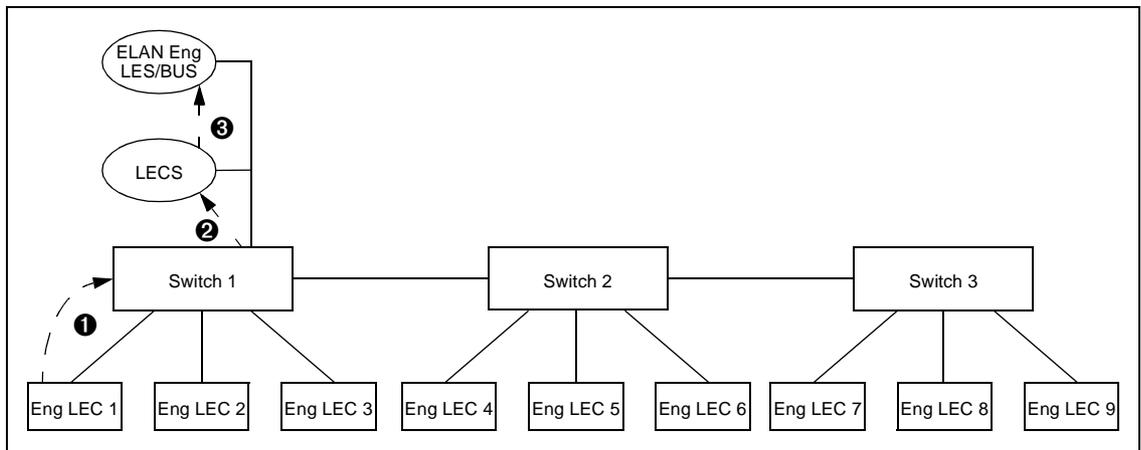
**Figure 7.12 - ELAN with Single Server and Multiple Switches Connecting to Services**
