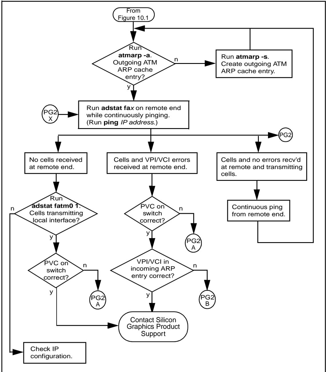
Figure 10.3 - Networking Connectivity Using PVCs (Page 1)
