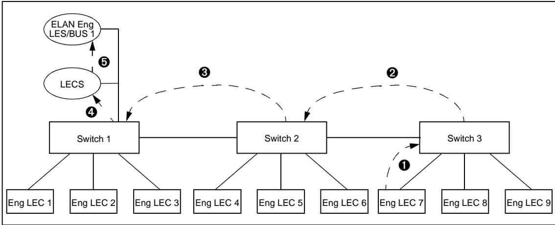
**Figure 7.13 - ELAN with Single Server and Remote Connection to Server**
