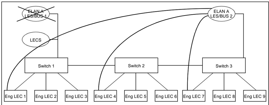
**Figure 7.18 - ELAN Re-established Using the Second Server**
