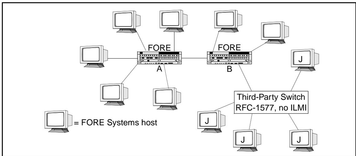
**Figure 6.2** - Configuring a Third-Party Switch with RFC-1577 and No ILMI Support
