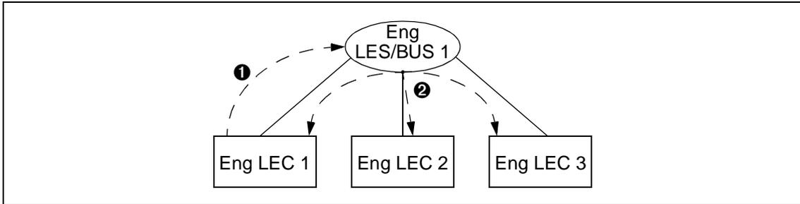
**Figure 7.4 - Broadcast IP-ARP Request**
