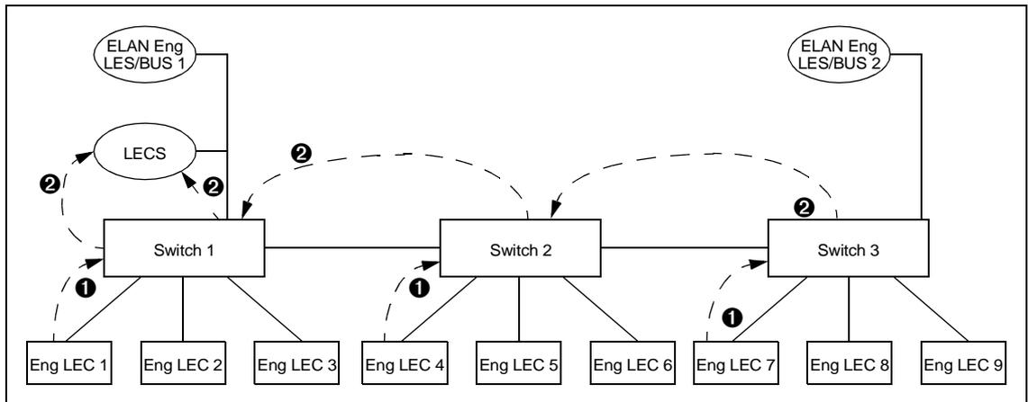
**Figure 7.15 - Registrations on an ELAN with Multiple Servers**
