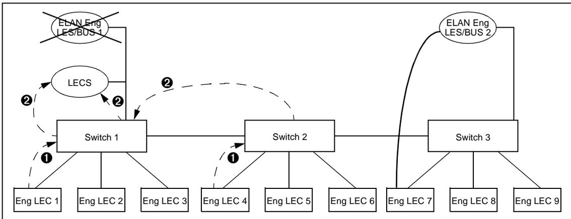
**Figure 7.17 - Failure of One ELAN Server and the Recovery Process**
