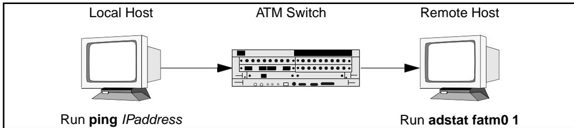
**Figure 10.2 - Hardware Configuration for Checking PVCs**
