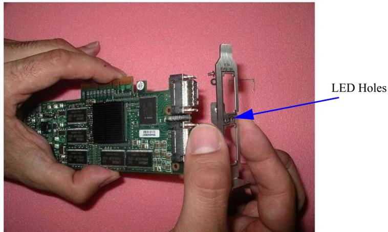
**short bracket to card** Insert a screw along with a washer into each of the two holes on the card intended for holding the bracket. Use a torque screwdriver to apply up to 2 lbs-in torque on each screw.
