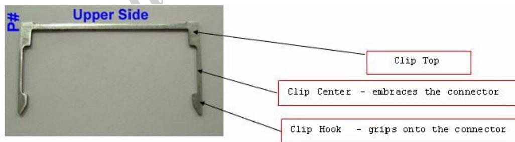
1. Using a small flat head screwdriver, gently push up one hook of a connector's clip toward the connector's top side as shown in Figure 9 (a) on page 30.
