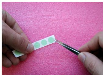
3. Gently place the label as shown in Figure 13. Make sure to align the center hole of the label with the drilled hole in the board.
