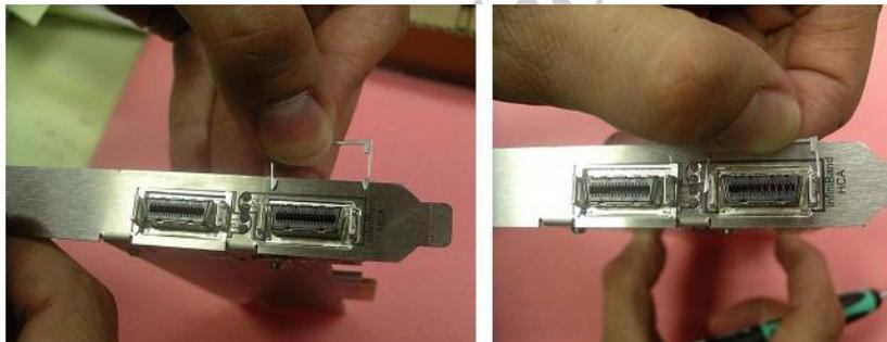
2. Use a small flat head screwdriver to gently slide the clip's hook towards the connector's base side as shown in Figure 19.
