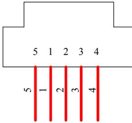
Table 1 - I2C-compatible Connector Pinout
