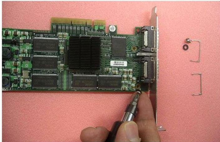
**Step 3 - Install Connector Clips** 1. Gently push one clip onto the connector. Make sure to slide both clip hooks (sides) around the connector evenly as shown in Figure 18.
