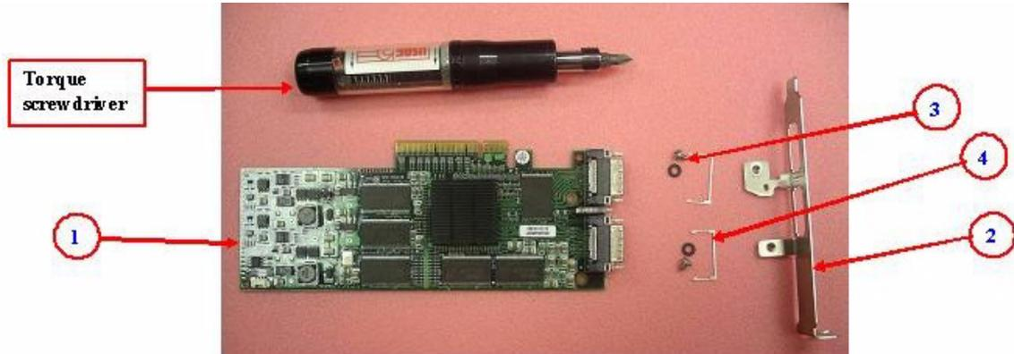
**Step 1 - Place short bracket onto card 5.** Gently place the bracket onto the card fitting the connectors through the bracket connector holes. Make sure the LEDs are aligned to their intended bracket holes. **Step 2 - Attach**
