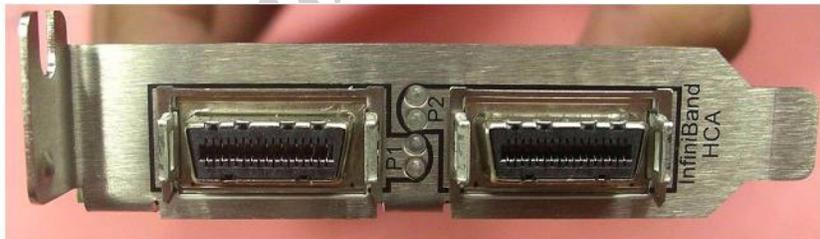
Figure 22: Print Side View After Short Bracket Assembly With Kapton Label
